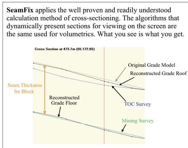
FIG 5 - SeamFix data view in cross-section.
