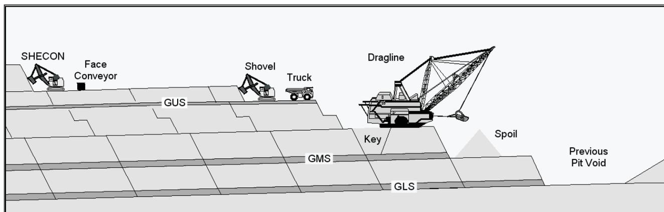
FIG 1 - Goonyella Riverside Mine stripping operations.
