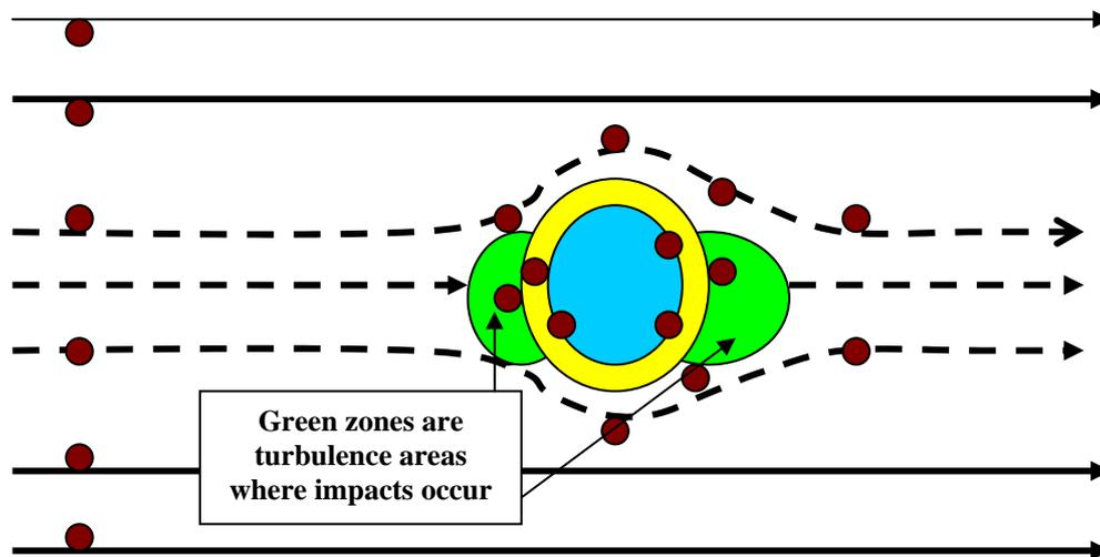
**Figure 5 – The turbulent areas around a water drop where impacts may occur (After “Beginners guide to Aeronautics”, NASA website, undated)**
