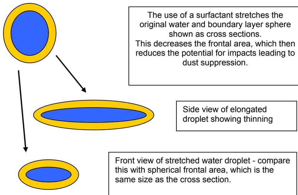
**Figure 6 – The effect of surfactant on a water droplet in airflow**
