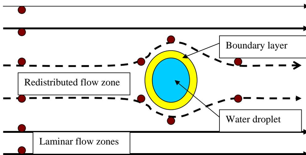
Figure 4 – The redistribution of laminar airflow around the boundary layer (After "Beginners guide to Aeronautics", NASA website, undated)
