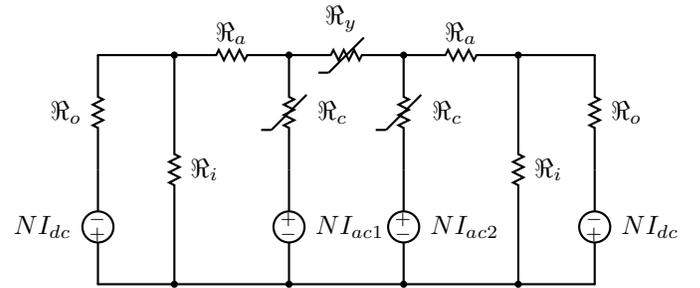
Fig. 10. Equivalent Open-Core Magnetic Circuit
