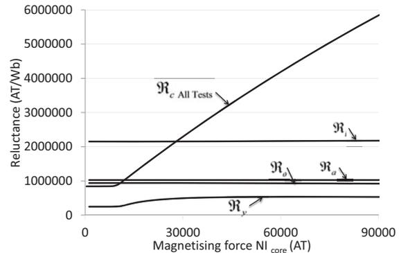
Fig. 17. Reluctance vs mmf of Relevant Flux Path
