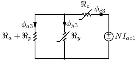
Fig. 11. Simplified Open-Core Circuit for Test 3
