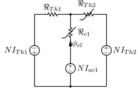
Fig. 19. Open-Core Circuit Reduction with  $\mathcal{R}_{c1}$  as load
