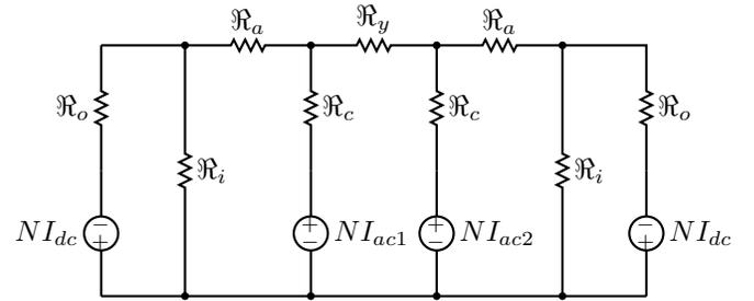
Fig. 3. Equivalent Magnetic Circuit
