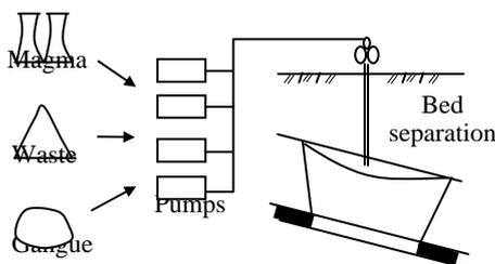
Figure 3 - Bed separation grouting technology under
