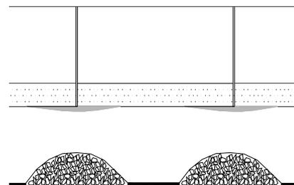
Figure 4 - Bed separation grouting the key strata
