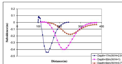
Figure 10 - Sensitivity analysis on panel width
