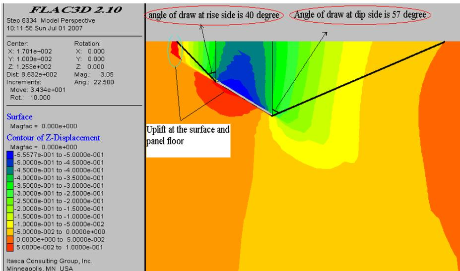
Figure 6 - Angles of draw at the sides of panel No 28 located at Madanjou coal mine
