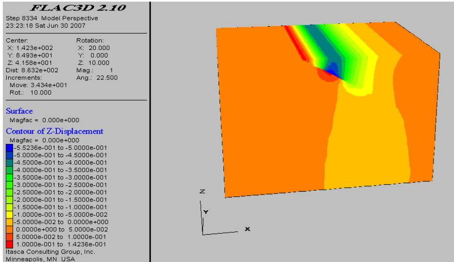
Figure 5 - Ground subsidence over panel No 28
