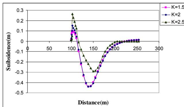
Figure 4 - Sensitivity analysis to initial stress
