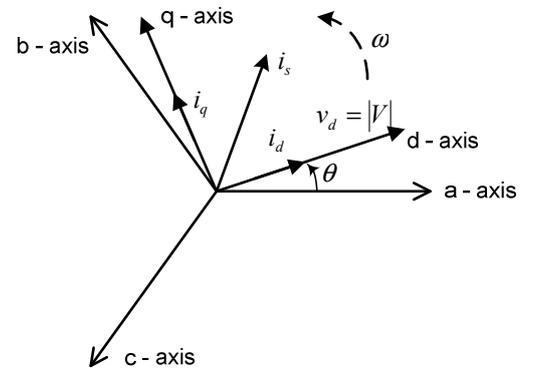
Fig. 2  $abc$  axes and the rotating reference frame  $dq$
