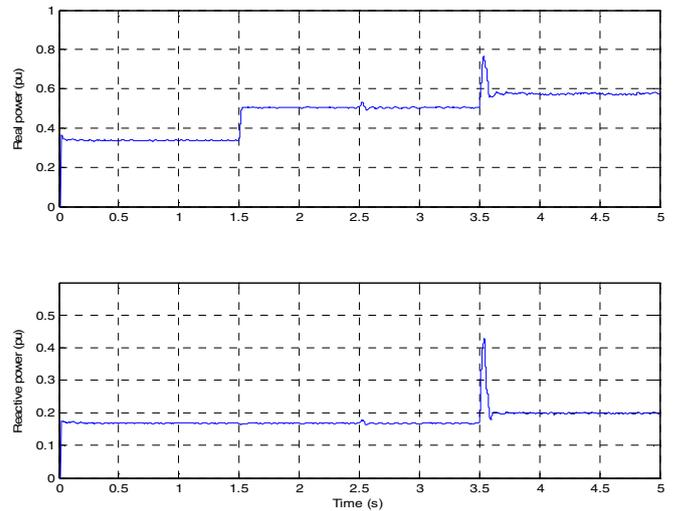
Fig. 8 Real and reactive power under varying wind and load conditions.
