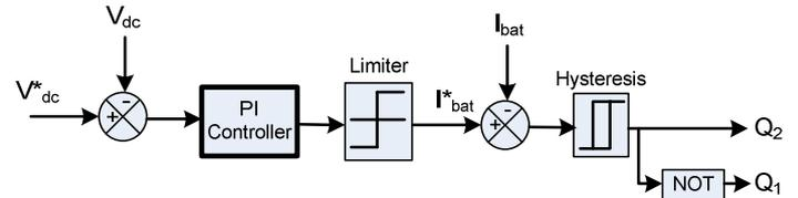
Fig. 5 Battery controller
