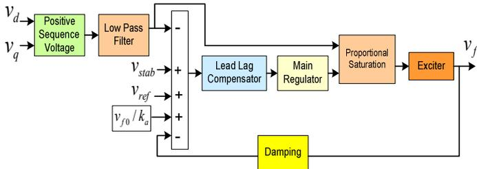
Fig. 4 IEEE Type 1 voltage regulator and exciter system
