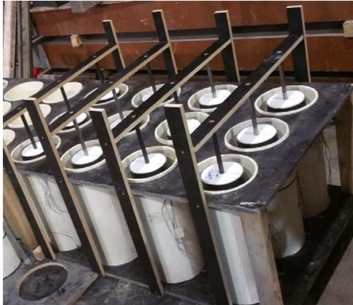
Fig. 4 Formwork for casting concrete
