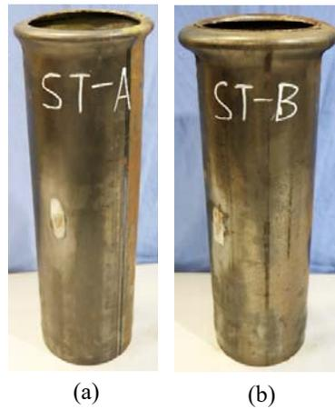
Fig. 2 Buckling mode of steel tubes:
