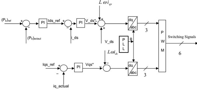
Fig. 6. Battery inverter controller
