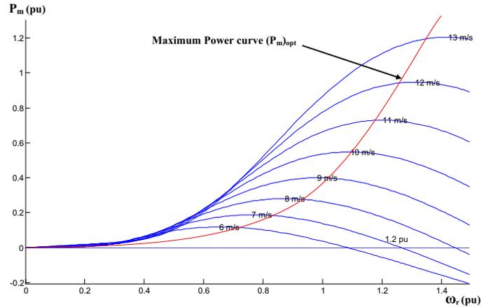
Fig. 2. Wind turbine power characteristics and maximum power extraction curve
