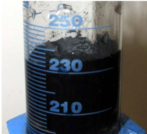
**Figure 4** Example of pulverised coal sticking to the inside of the glass tube above the water layer
