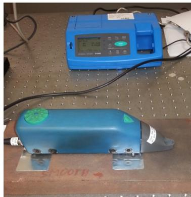
**Figure 2** Hommel T1000 surface roughness tester
