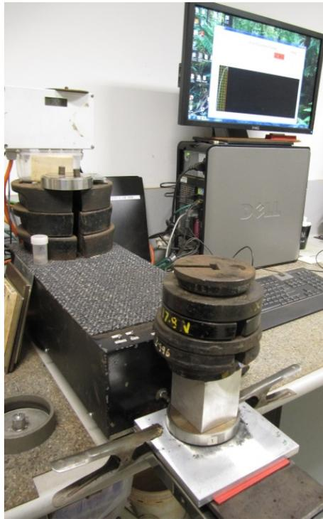
**Figure 5** The translational shear tester (TST) used in this test program
