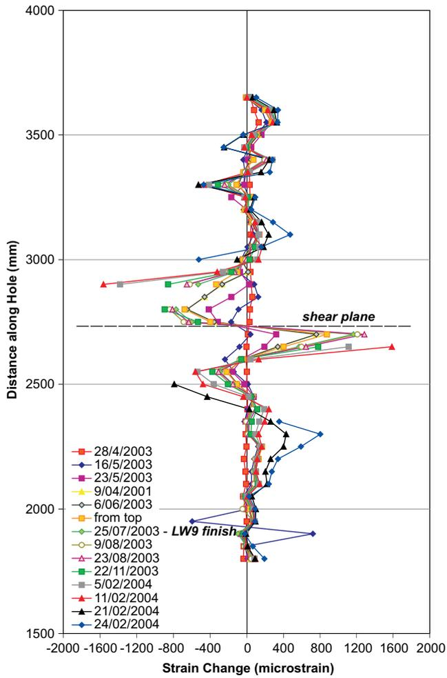
FIG A3 - Strain change on chain pillar side after extraction of Longwalls 9 and 10.
