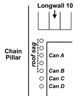
FIG 13 - Views of tailgate looking inbye – roof conditions on block side of supports significantly better than chain pillar side.
