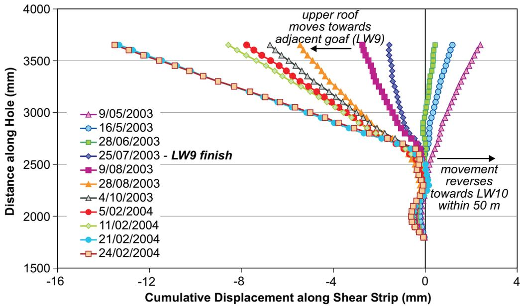
FIG A2 - Cumulative displacement along shear strip – block side during extraction of Longwalls 9 and 10.
