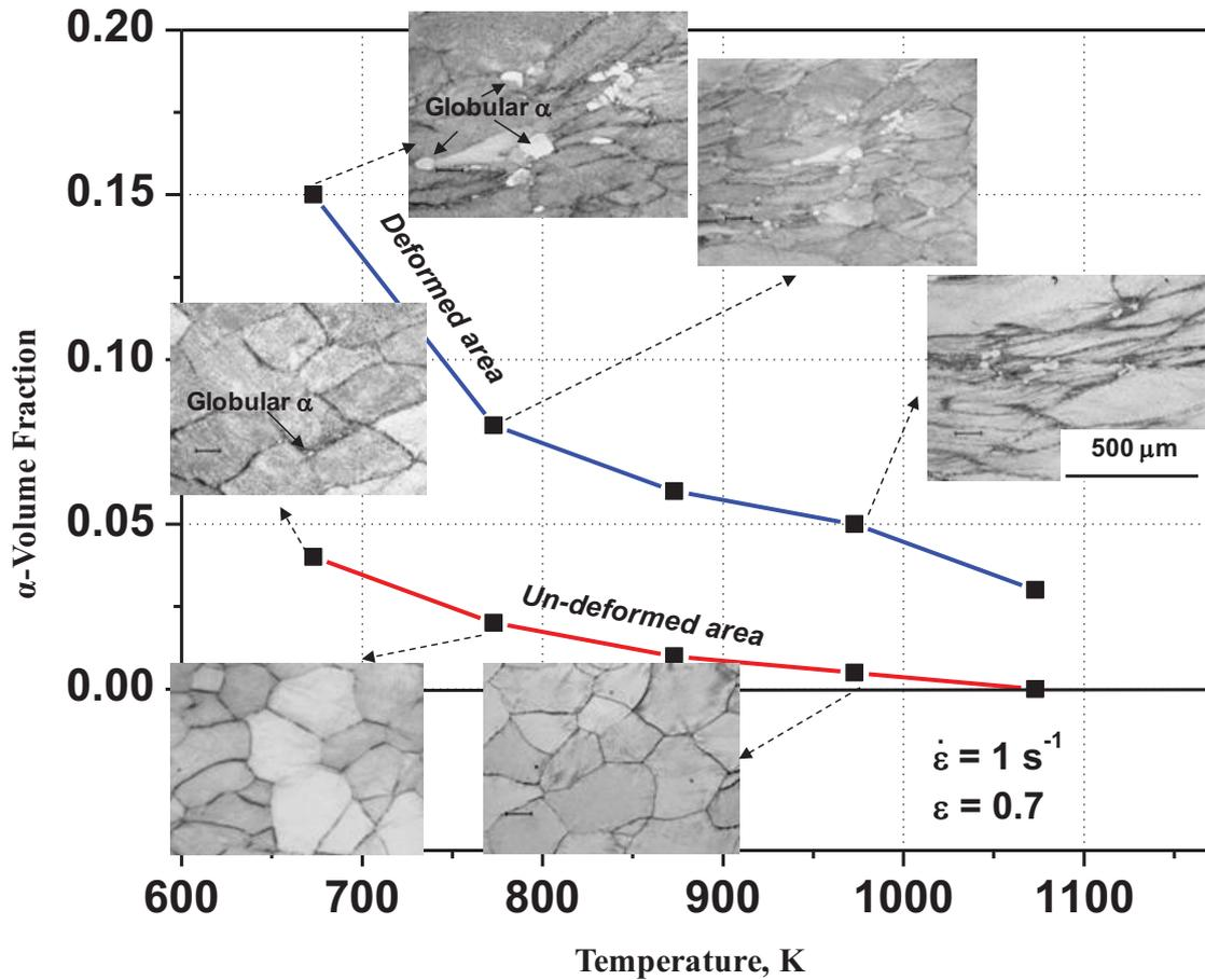
Figure 4 Effect of slow cooling on the volume fraction of  $\alpha$  and the morphology of deformed and un-deformed samples
