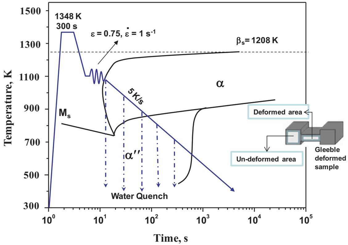
Figure 1 Thermo-mechanical schedules superimposed on a schematic TTT diagram of the Ti-6246 alloy
