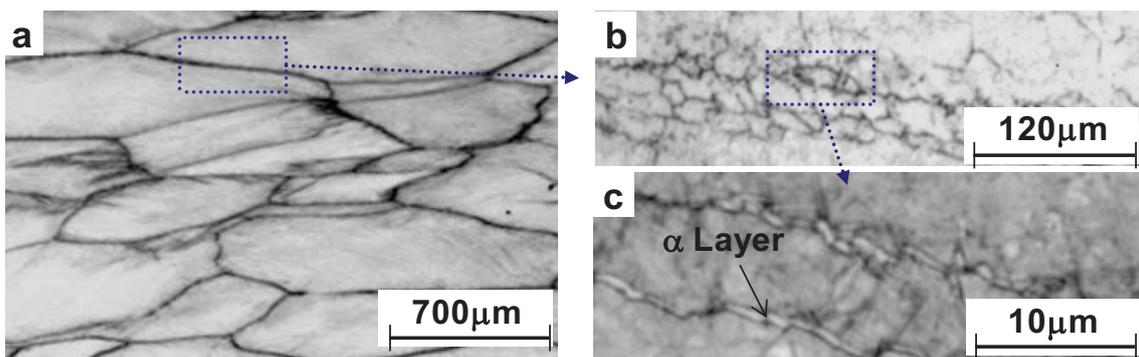
Figure 5 a) Formation of  $\alpha$ -layers on  $\beta$  grain boundaries after deformation at 1075 K, cooling to 873 K and water quenching. b) DRX on  $\beta$ - grain boundaries during deformation and c) Formation of  $\alpha$ -layers on recrystallized  $\beta$ - grain boundaries.
