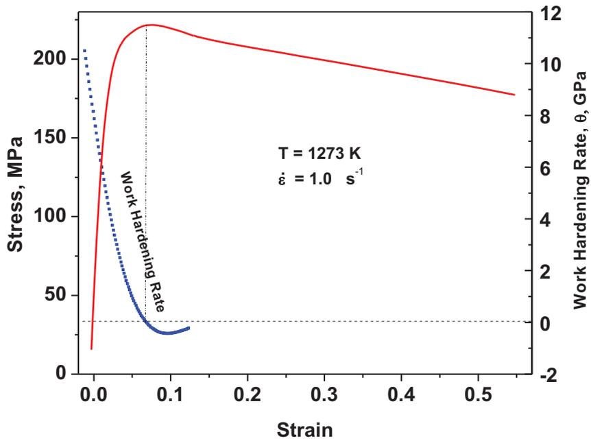
Figure 2 Typical stress-strain curve and work hardening rate of a Ti-6246 alloy following prior deformation at 1073 K and a strain rate of  $1 \text{ s}^{-1}$
