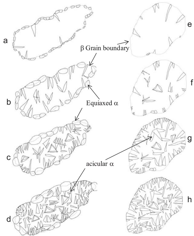
Figure 6 Schematic figure of microstructure development during slow cooling of a deformed (a-d) and un-deformed (e-h) Ti-6246 sample
