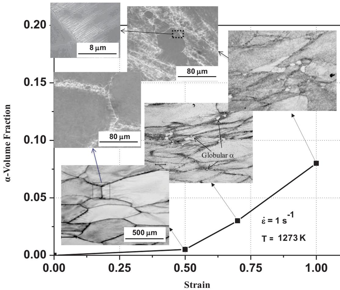
Figure 3 Effect of deformation on the volume fraction and morphology of the  $\alpha$ -phase
