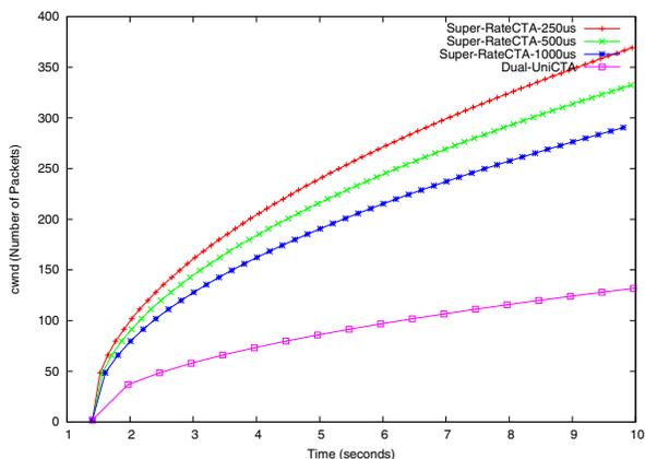
**Figure 2.** This shows the effect of a 5ms time block being broken up into blocks of 250 $\mu$ s, 500 $\mu$ s, 1000 $\mu$ s and 5000 $\mu$ s. The Imme-ACK policy was used in this experiment.
