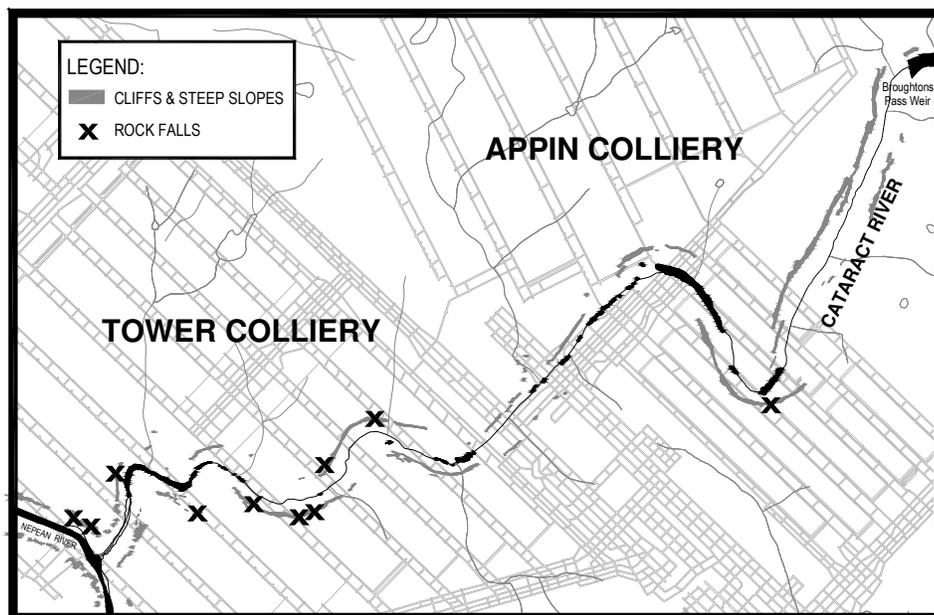
Fig. 6 – Observed rock falls over Tower Colliery
