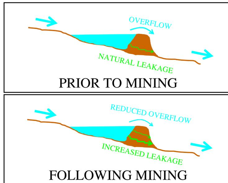
**Fig. 4 - Diagrammatic Representation of Rockbar Leakage**
