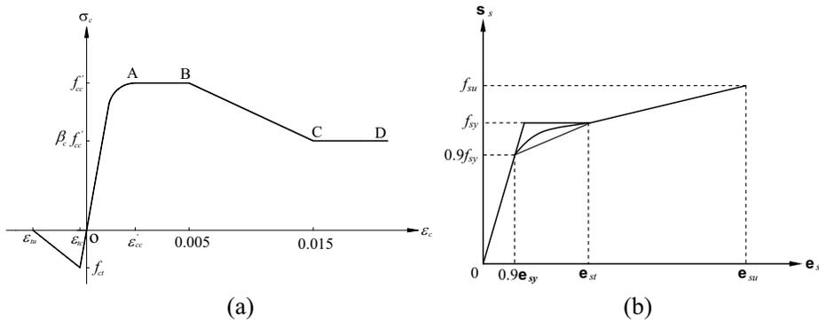
Figure 2: Material models: (a) Concrete (b) Structural steels
