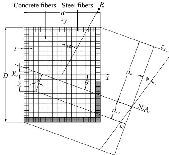
Figure 1: Fiber element discretization of CFST column section
