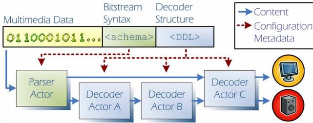
**Fig. 1.** A general view of an RMC bitstream
