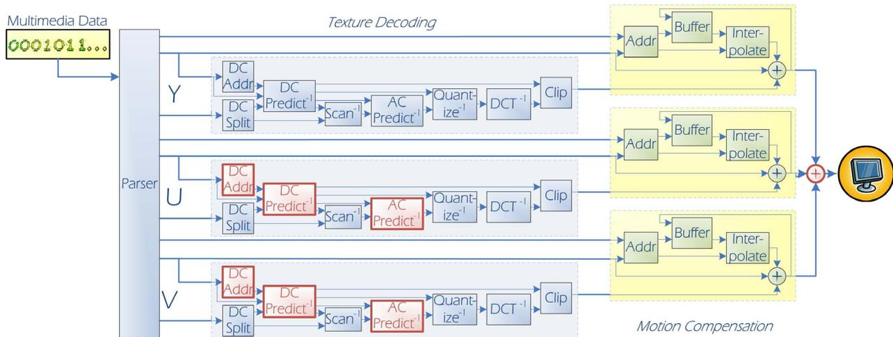
Fig. 4. MPEG-4 Video Simple Profile decoder & extensions
