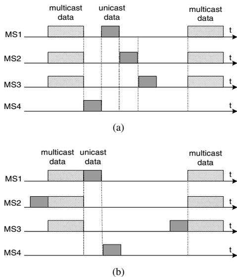
Fig. 1. Scheduling Samples for unicast and multicast traffic
