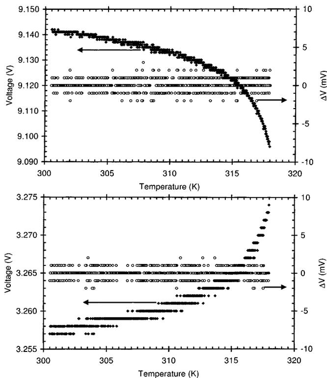
Fig. 2. Control experiment without radiation, showing the changes versus temperature of the measured, absolute threshold voltages  $V_{th}$  (filled circles) and the “dose signal”  $\Delta V_{th}$  (open circles) provided by the CMRP-designed reader system. Shown for the two types of p-MOSFET on the REM Type TOT502 (top figure) thick oxide, Type R and (bottom figure) thin oxide, type K. No temperature-related trend is evident in the  $\Delta V_{th}$  data, only ADC noise.
