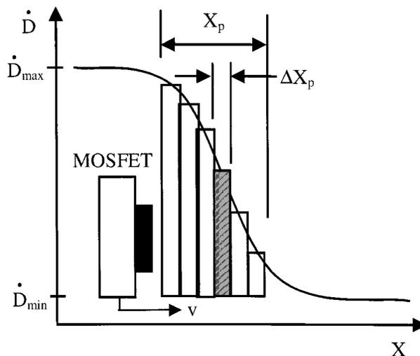
Fig. 3. Schematic representation of a penumbra dose rate versus distance. The width of the penumbra is  $X_p$  and the spatial resolution of the MOSFET sensor is  $\Delta X_p$ .
