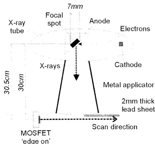
Fig. 5. Penumbra formation of the Siemens X-ray machine.
