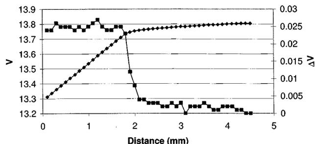
Fig. 7. Online measurement with an "edge-on" TOT500 RADFET of the penumbral profile formed by a lead plate in the beam of 120-kV<sub>p</sub> X-rays, using the setup shown in Fig. 5.
