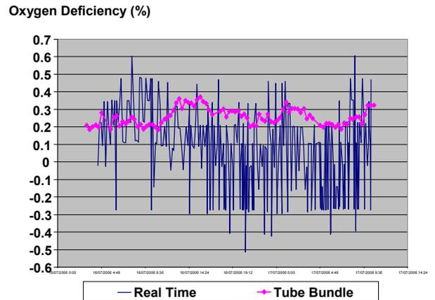
Figure 2 - Real time vs tube bundle oxygen deficiencies
