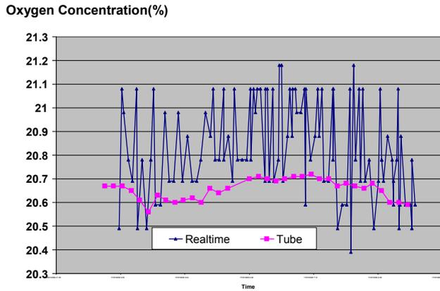
Figure 1 - Real time vs tube bundle oxygen measurements
