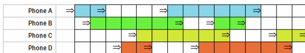
Figure 4f. An automated event sequence determines when sound is produced on each phone. Every 15-30 seconds an event occurs, i.e. a single tone either starts or stops.
