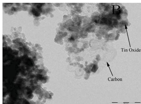
Figure 1, (A) SEM image of sample after hydrochloric acid treatment, (B) TEM image of tin-rich particles dispersed in the nano-carbon matrix.
