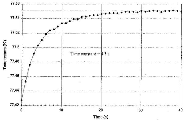
Fig. 5. Calorimeter performances for a temperature increase.
