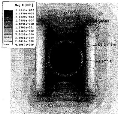
Fig. 7. Field map generated in the solenoid.
