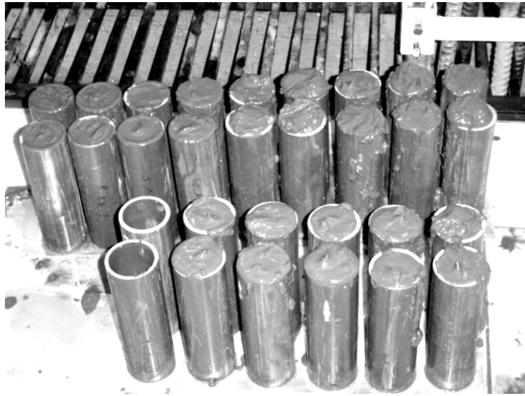
Figure 2 - Grout samples poured for mechanical properties tests.
