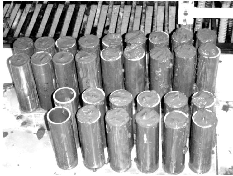
Figure 2 - Grout samples poured for mechanical properties tests.
