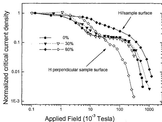
Fig.2 Normalised magnetic dependence of transport  $J_c$  at 77 K for three samples with deformation rates 0 %, 30 % and 80 %, respectively.
