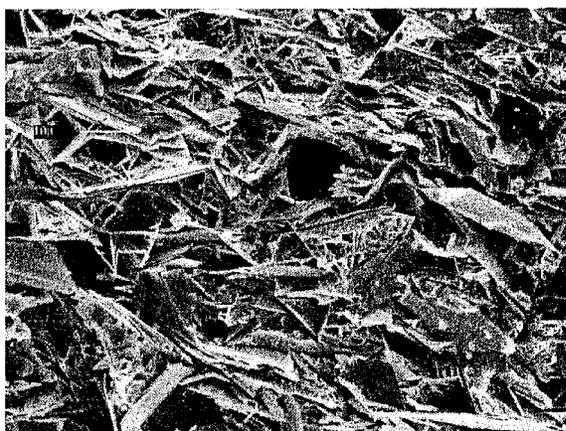
Fig. 4 (b) A SEM image of the fractured cross section for a sample with a deformation rate of 60 %.
