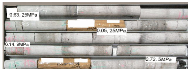
Figure 7 - Core photograph showing Axial PLT, inferred UCS and Diametral PLT Is50 values
