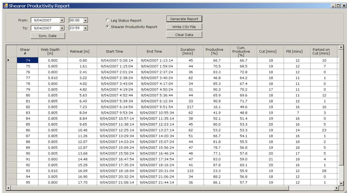
Figure 9 - Screen dump of shearer production report
