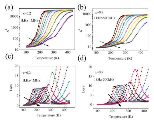
FIG. 2. (Color online) Temperature dependence of the real dielectric constants and loss for representative samples.
