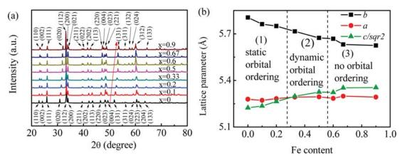
FIG. 1. (Color online) (a) X-ray diffraction patterns of all samples, (b) x dependence of lattice parameters.
