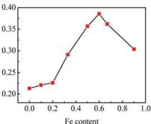
FIG. 5. (Color online) Fe content dependence of characteristic frequency  $f_0$  (left) and activation energy  $E_{\alpha}$  (right).
