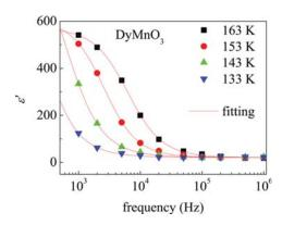
FIG. 3. (Color online) Frequency dependence of the real dielectric constant  $\varepsilon'$  at various temperatures: scattered symbols, experimental data; lines, the output of fitting via the modified Debye equation.
