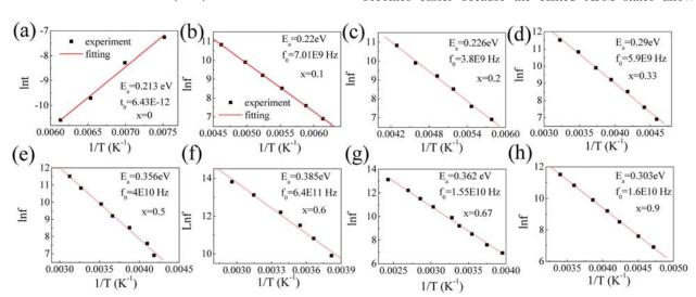
FIG. 4. (Color online) Arrhenius law fitting for all samples and corresponding activation energies at low temperature.
