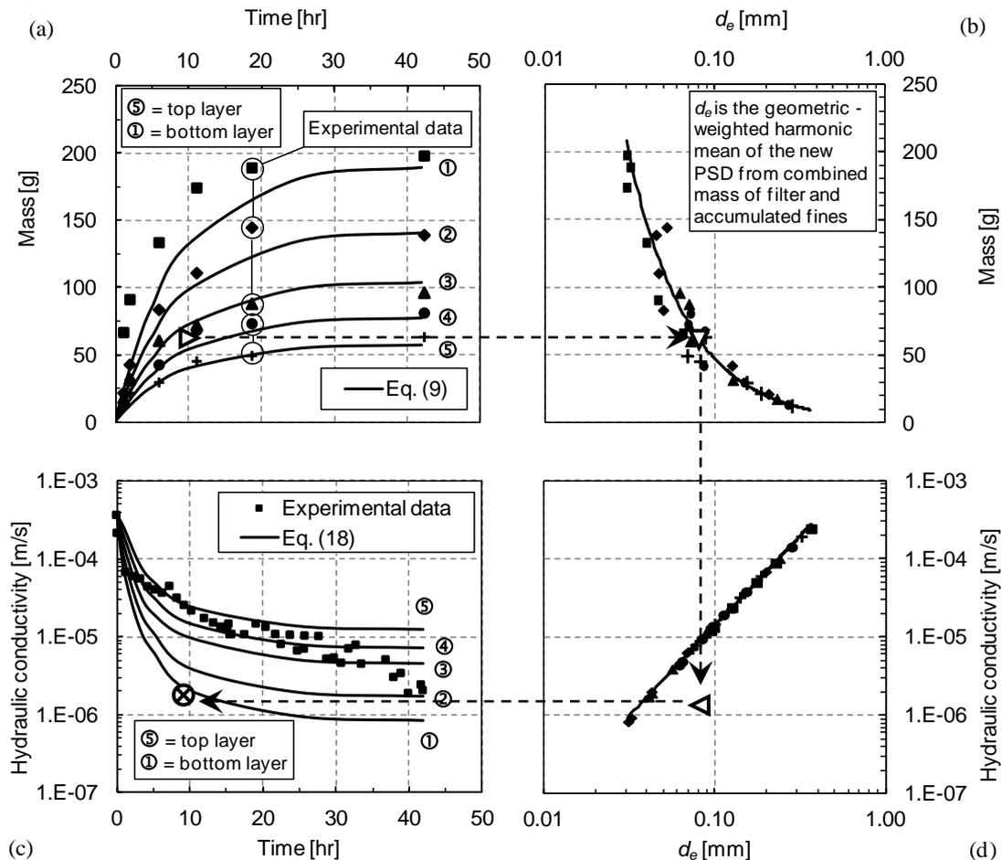
Figure 4: Porosity based family of curves generated from Eqs. (1) to (17); circled numbers represent the filter layers;  $n_0 = 34.96\%$ ,  $k_0 = 3.66 \times 10^{-4}$  m/s,  $\epsilon_f = 0.009$ ,  $V_0 = 1.44 \times 10^{-3}$  m<sup>3</sup>,  $\rho_a = 2,700$  kg/m<sup>3</sup>,  $N_{max} = 763,500$  cycles,  $f = 5$  Hz.
