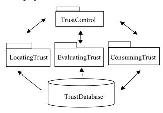
Fig.3. TrustEngine Package Hierarchy
