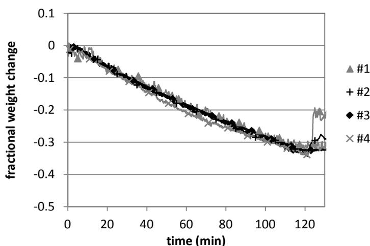
Figure 2. Fractional weight change curves for coke analogue samples with no mineral matter, fired at 1600°C, reacted with CO<sub>2</sub> at 1100°C for 120 minutes.
