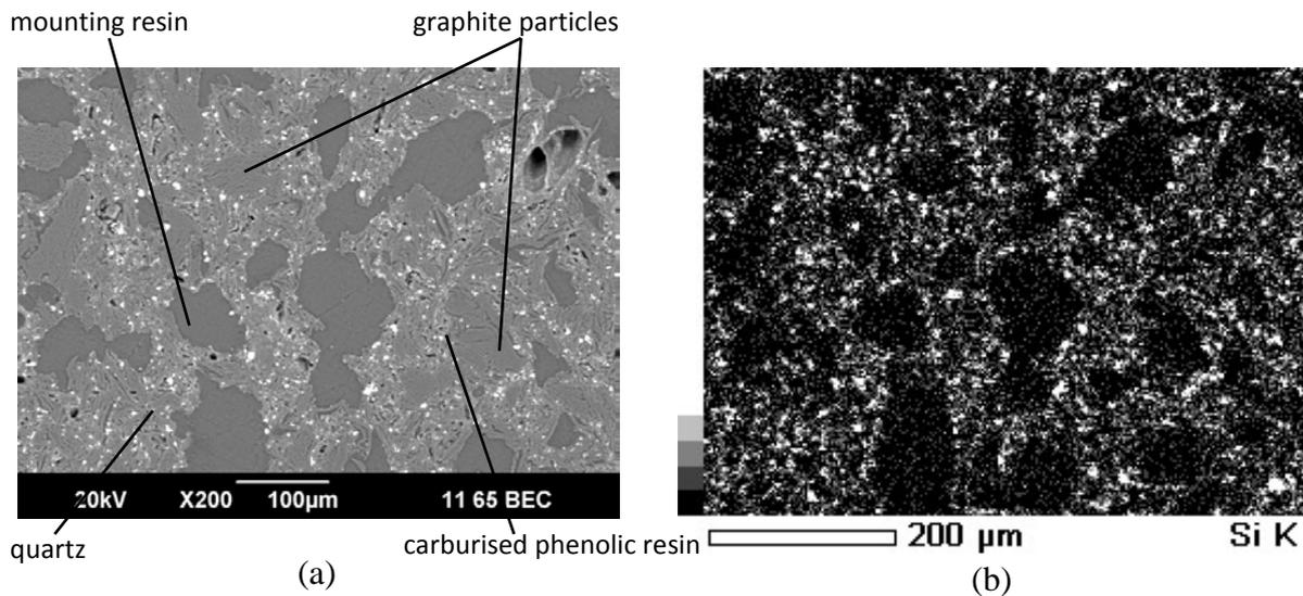
Figure 5. SEM image and EDS elemental map for a coke analogue sample containing 0.1 mol/100g quartz. (a) Typical field of view at low magnification; (b) Si elemental map.
