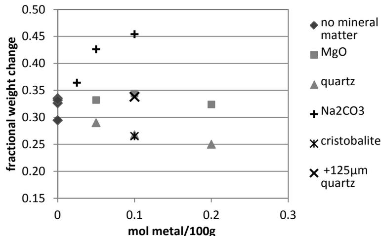
Figure 4. The final fractional weight change of the coke analogue samples after reaction with CO<sub>2</sub> at 1100°C for 120 minutes.
