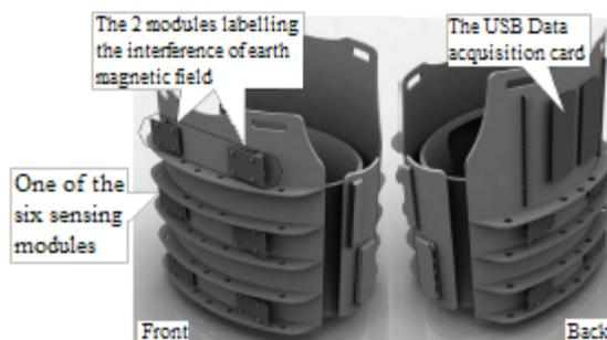
Fig. 3. Wearable sensing modules by Wu *et al.* [42].
