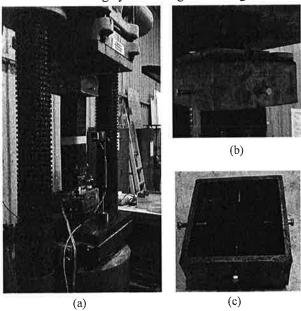
Figure 3. (a) Loading system (b) Loading head and overhang edges (c) Loading head
