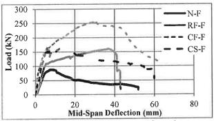
Figure 11. Load-midspan deflections plot of flexural tests
