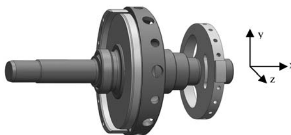
Fig. 12 Balanced shaft and its associated parts assembly
