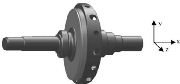
Fig. 11 Three-dimensional drawing of the unbalanced shaft assembly
