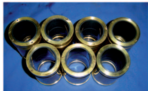
Fig. 10 Picture of sleeves with CFRP liner
