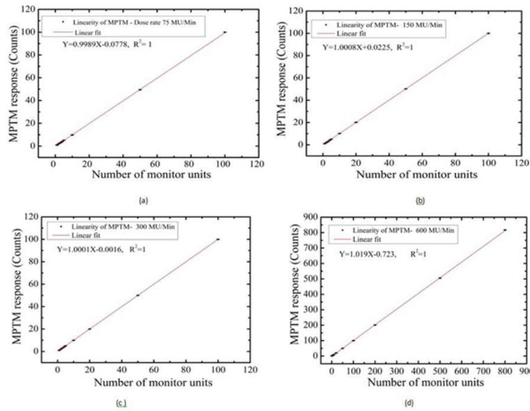
**Figure 1.** MPTM central detector response vs dose with different linac pulses frequency for 6 MV photon beam and 10x10 cm<sup>2</sup> field size.
