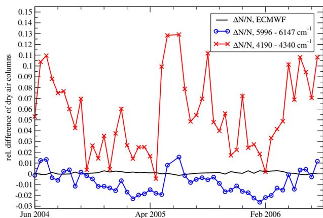
**Fig. 4.** Impact of spectroscopic line lists on derived pressure at Park Falls. Black: total dry air column for fixed ECMWF pressure profile, plotted as relative difference to in-situ measurement. Circles: dry air column derived from 5996–6145 cm<sup>-1</sup>, crosses: dry air column derived from 4190–4340 cm<sup>-1</sup>.
