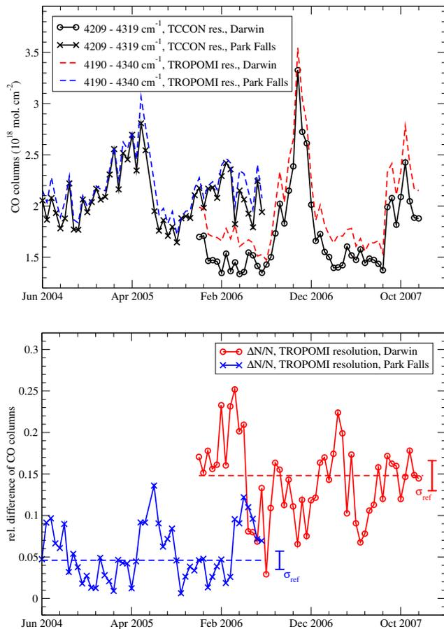
**Fig. 6.** CO retrieval accuracy at 4190–4340 cm<sup>-1</sup> for Darwin (circles) and Park Falls (crosses). The upper panel shows the time-series, the lower panel shows the relative differences between columns retrieved at TROPOMI resolution and columns retrieved from window 5 (original high resolution).
