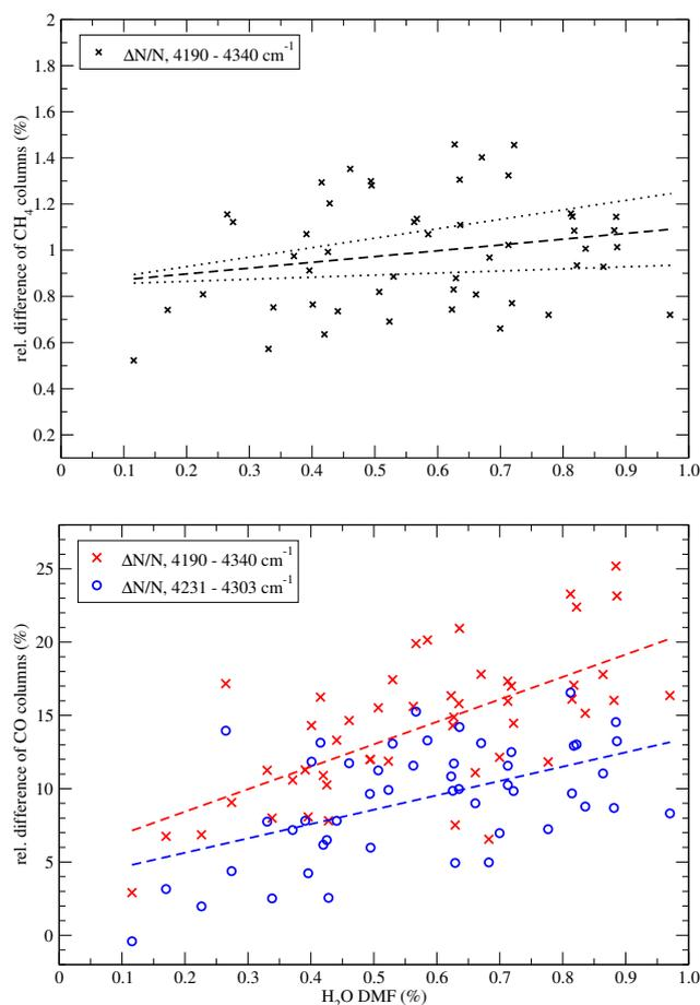
**Fig. 8.** Correlation of retrieval errors with humidity at Darwin. Deviations of CH<sub>4</sub> (upper panel) and CO columns (lower panel) with respect to the reference values are plotted against H<sub>2</sub>O DMF. Red crosses indicate nominal CO retrievals, blue circles show results for an optimised CO sub-window. Dashed lines denote linear fits.
