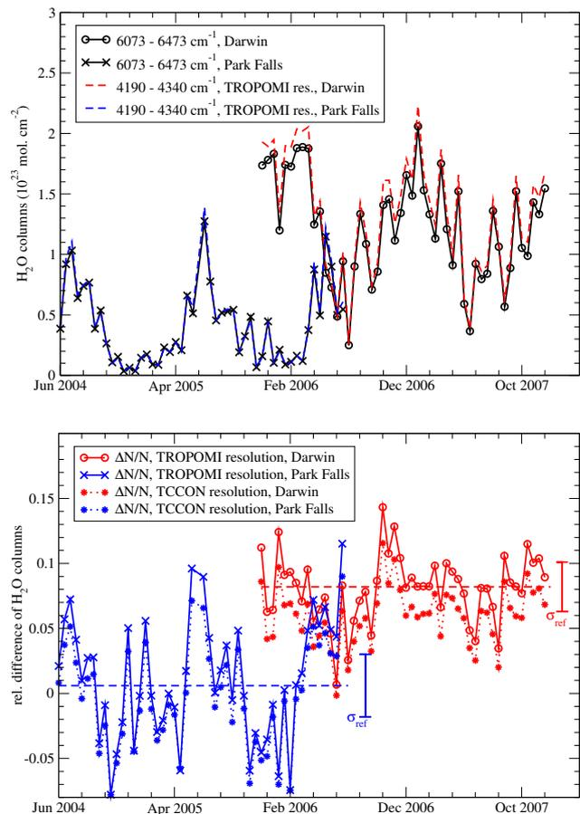
**Fig. 7.** H<sub>2</sub>O retrieval accuracy at 4190–4340 cm<sup>-1</sup> for Darwin (circles) and Park Falls (crosses). The upper panel shows the time-series, the lower panel shows the relative differences between columns retrieved at 4190–4340 cm<sup>-1</sup> (for TROPOMI and original high resolution) and columns retrieved from window 4.
