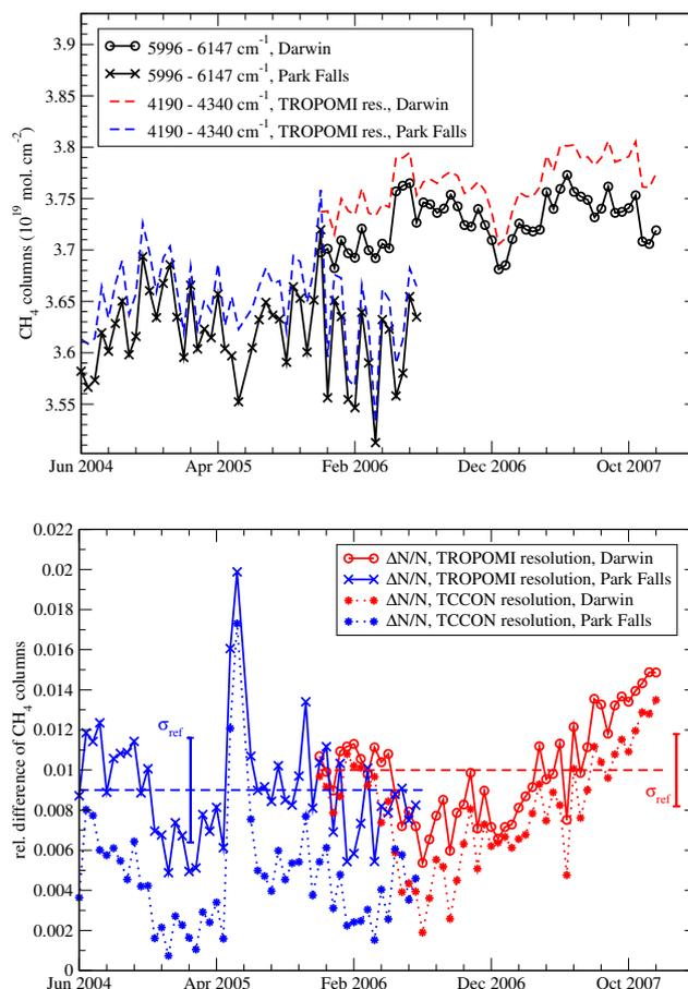
**Fig. 3.** CH<sub>4</sub> retrieval accuracy for the 4190–4340 cm<sup>-1</sup> range. The upper panel shows the time-series of CH<sub>4</sub> columns at Park Falls (crosses) and at Darwin (circles). The lower panel shows the relative differences between columns retrieved at original (dotted lines) and at TROPOMI resolution (solid lines) with respect to reference values from 5996–6145 cm<sup>-1</sup>.
