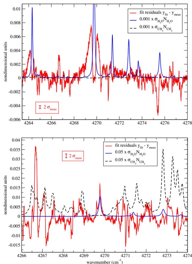
**Fig. 5.** Spectral fit residuals for wet atmospheric conditions at Darwin (upper panel) and for dry atmospheric conditions at Park Falls (lower panel). Fit residuals (red line) are over-plotted with optical depth of H<sub>2</sub>O (blue line) and CH<sub>4</sub> (black dashed line), average measurement uncertainty indicated by error bars in boxes.
