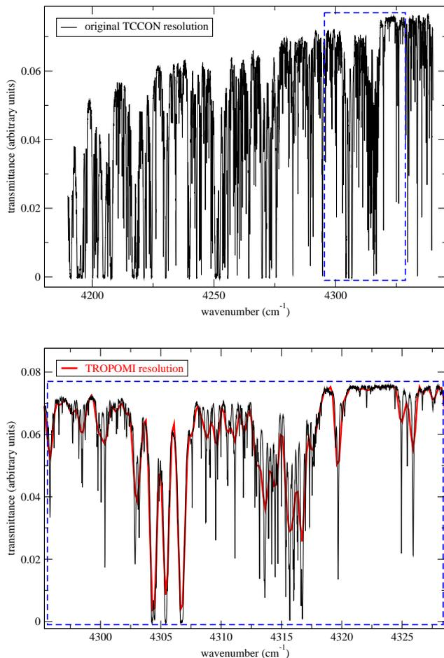
**Fig. 1.** Upper panel: original TCCON spectrum of the TROPOMI wave number range 4190–4340 cm<sup>-1</sup>, measured at Darwin. Lower panel: magnification of the 4300–4325 cm<sup>-1</sup> range (blue dashed box) with both the original spectrum (black) and the same spectrum, convolved with the TROPOMI instrument response function (red).
