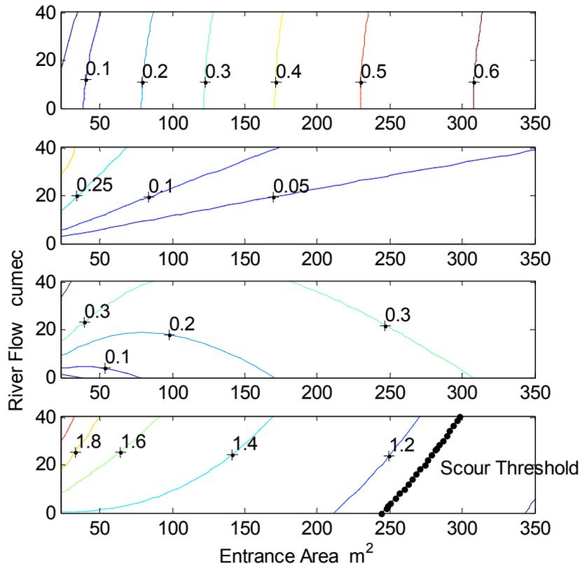
Figure 4 Contours of a) Tidal amplitude, b) Mean tidal level, c) Maximum water level, d) Maximum ebb velocity - non-scouring to right of line. Parameters based on Snowy River late September 2008
