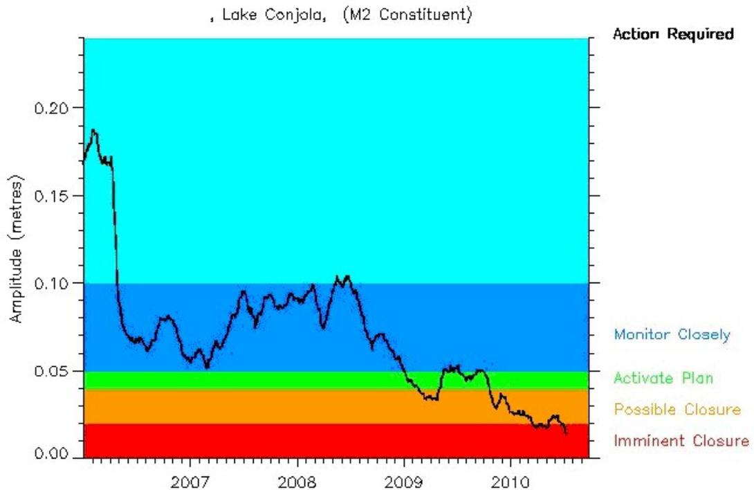
**Figure 2** Screen capture of the DST display for Lake Conjola (Source: Manly Hydraulics Laboratory, NSW <http://www.mhl.nsw.gov.au/www/lconj.htmlx>)
