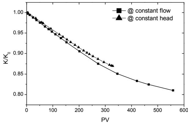
Figure 4. Normalised hydraulic conductivity vs. pore volume
