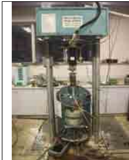
Figure 3. Large-scale cylindrical triaxial apparatus.
