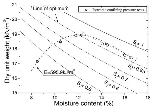
Figure 2. Compaction curve for the standard energy level.
