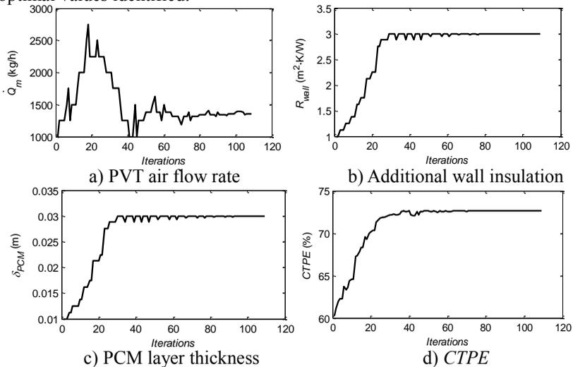
Fig. 4 Optimization process when using the Hooke-Jeeves pattern search method.
