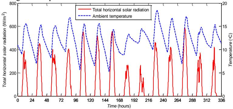
Fig. 2 Solar radiation and ambient air temperatures during the 14 winter test days.
