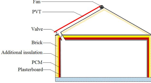
Fig. 1 Illustration of the PCM-enhanced house with PVT collectors on the roof.
