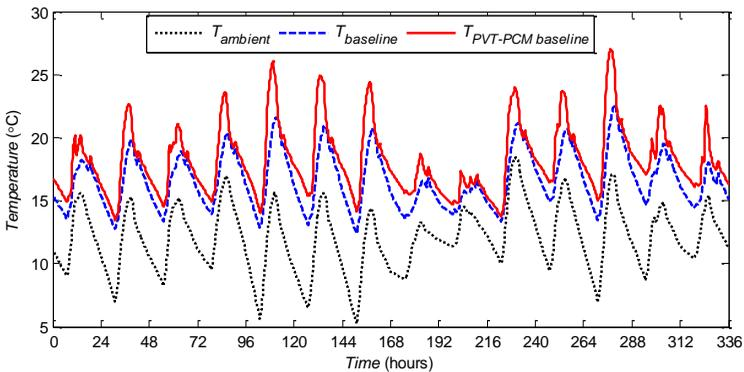
Fig. 3 Indoor temperature of the house under the PVT-PCM baseline case and baseline case without using PVT collectors and PCMs for building thermal management.
