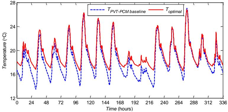
Fig. 5 Indoor temperatures of the PCM-enhanced house with integrated air-based PVT collectors by using the optimal design, and the house under the PVT-PCM baseline case without optimization.
