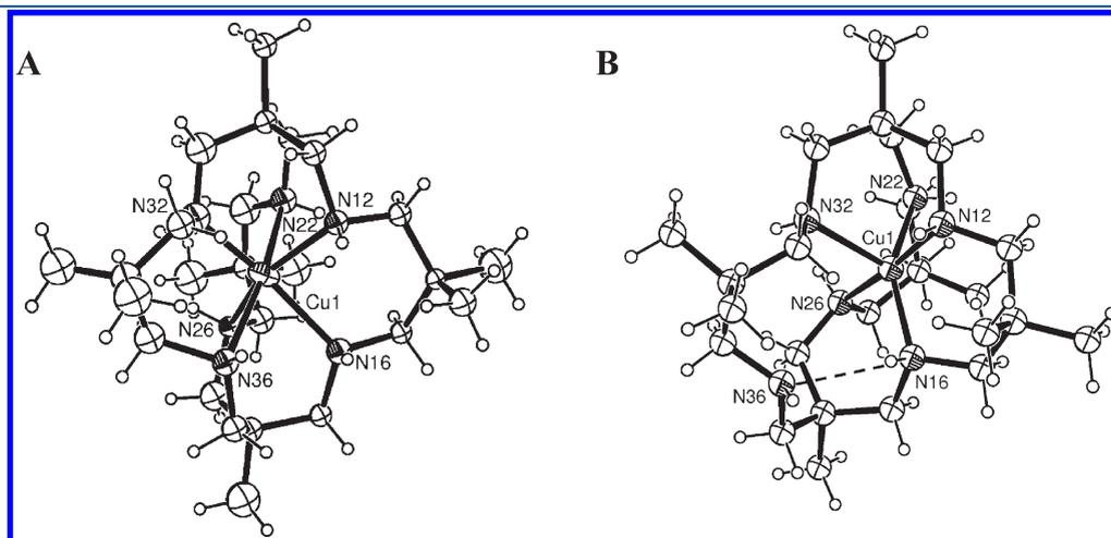
**Figure 2.** ORTEP views (from the same aspect) of (A) six-coordinate [Cu(Me<sub>8</sub>tricosaneN<sub>6</sub>)](NO<sub>3</sub>)<sub>2</sub>·2H<sub>2</sub>O and (B) five-coordinate [Cu(Me<sub>8</sub>tricosaneN<sub>6</sub>)](S<sub>2</sub>O<sub>6</sub>). 30% probability ellipsoids are shown, and anions have been omitted for clarity. Note the same configuration of the coordinated N-donors is present in both complexes while a H-bond to N36 in B replaces the coordinate bond in A.
