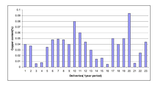
Figure 1 Variation in copper content (% Cu) of welding wires delivered in 23 shipments over a 1 year period. [20]
