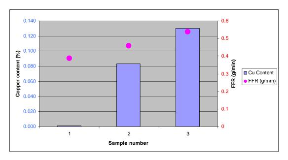
Fig 3 Fume formation Rate results versus copper content of sample wire
