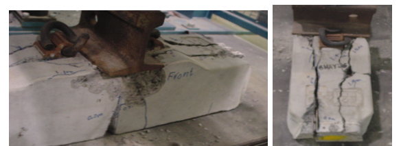
d) impact failure at 1,600 kN
