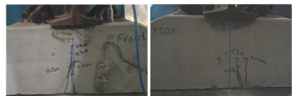
b) impact forces between 700 and 1,000 kN
