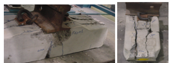
d) impact failure at 1,600 kN
