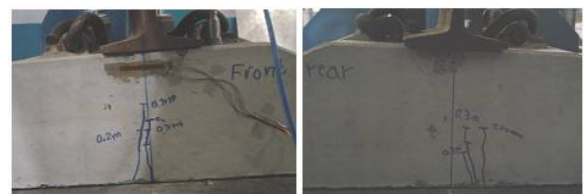
a) impact forces between 150 and 600kN
