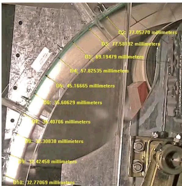
**Figure 6a** Material stream height through the hood
