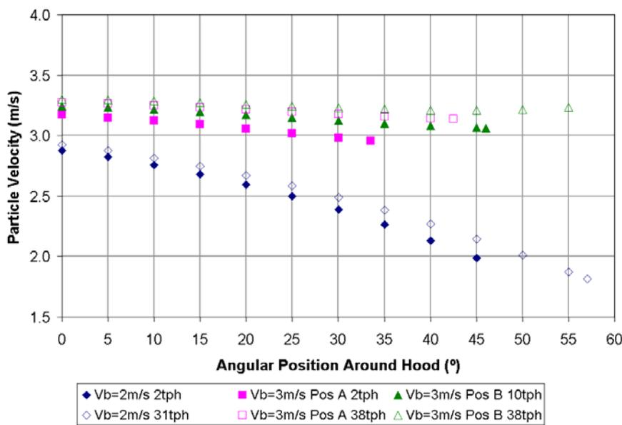
**Figure 10** Predicted stream velocity through hood by Korzen method
