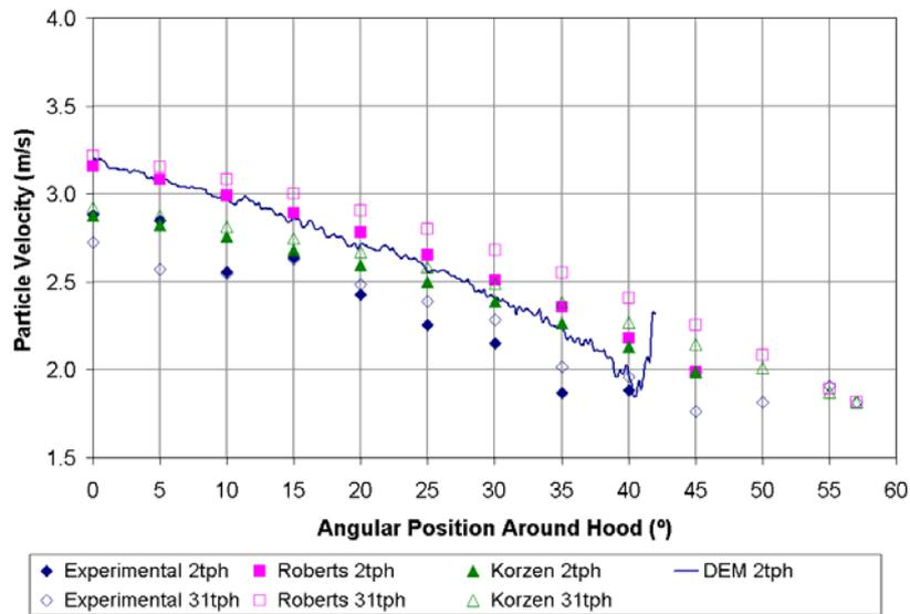
**Figure 14** Comparison of methods for a belt speed of 2m/s
