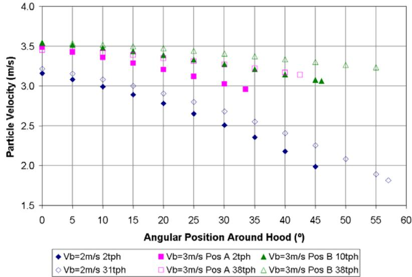
**Figure 8** Predicted stream velocity through hood by Roberts method
