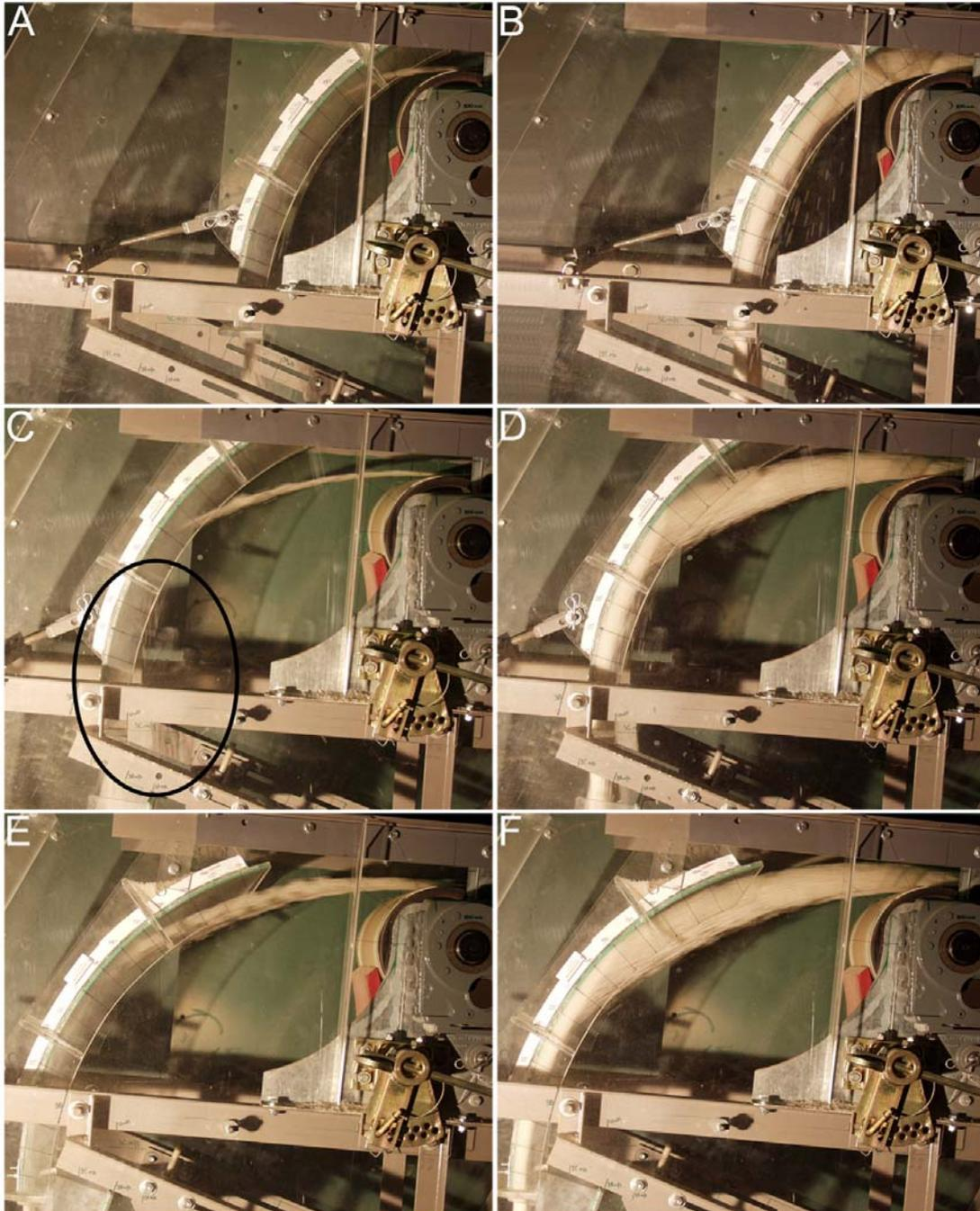
**Figure 3** Material flow through the conveyor hood
