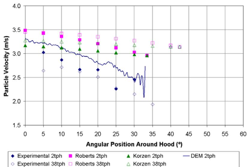
**Figure 15** Comparison of methods for a belt speed of 3m/s with the hood in position A
