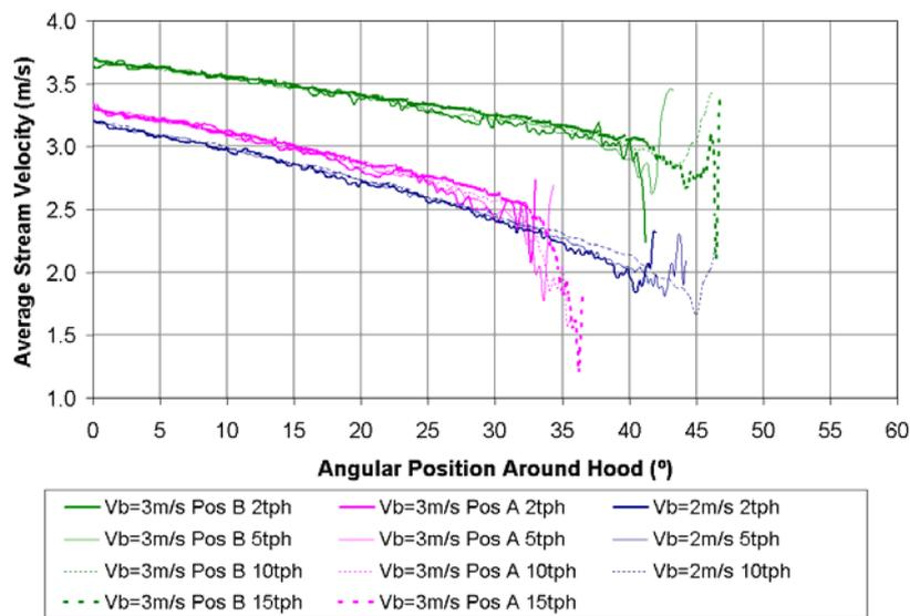
**Figure 13** DEM simulation results for all material feed rates
