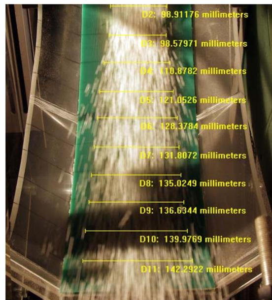
**Figure 6b** Material stream width through the hood
