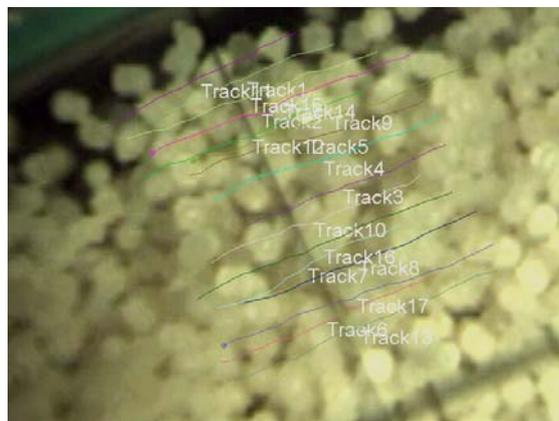
**Figure 4** Particle tracking using Image Pro Plus
