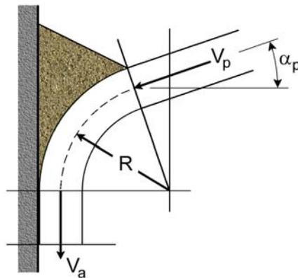
**Figure 9** Flow representation for analysis by Korzen
