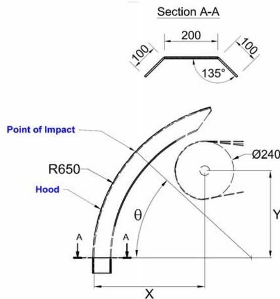
**Figure 2** Detail of conveyor transfer hood
