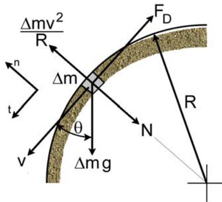
**Figure 7** Force diagram for the inverted curved chute
