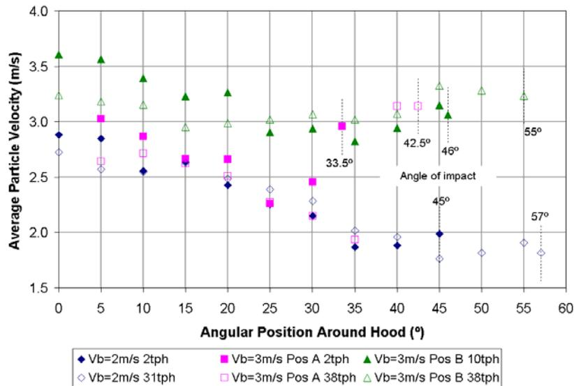
**Figure 5** Average particle velocity at each angular position around transfer hood
