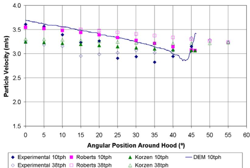
**Figure 16** Comparison of methods for a belt speed of 3m/s with the hood in position B
