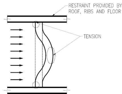
Figure 2: Plate mechanism (Pearson)
