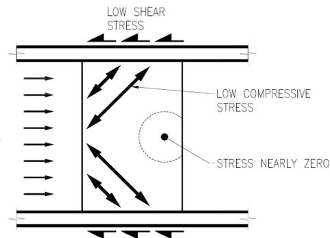
Figure 4: Plug mechanism
