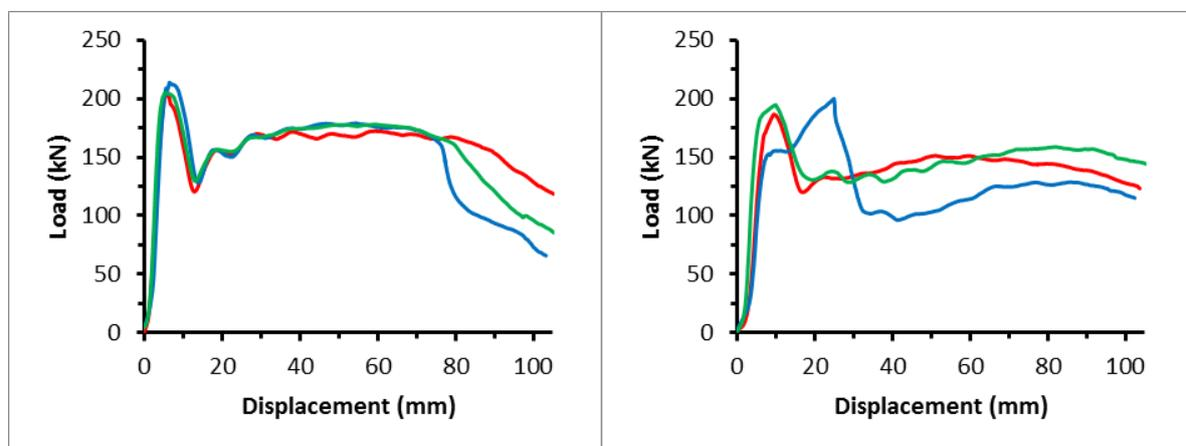
Figure 6: Results of testing with a 62 MPa grout in a 42 mm (left) and 52 mm (right) diameter borehole
