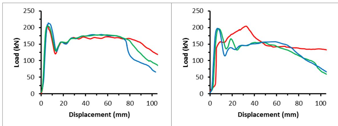
**Figure 9: Results of testing in standard borehole of 42 mm with a 62 MPa grout (left) and 80 MPa grout (right)**
