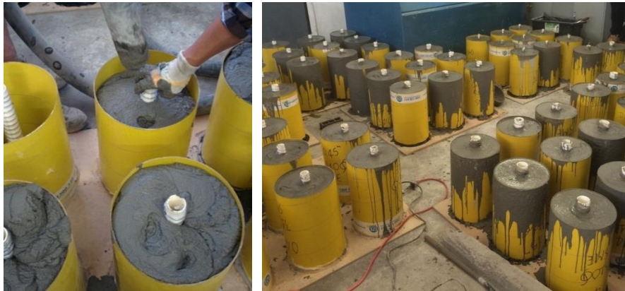
Figure 5: Cement-based material being pumped into moulds (left) and, samples immediately after casting (right)
