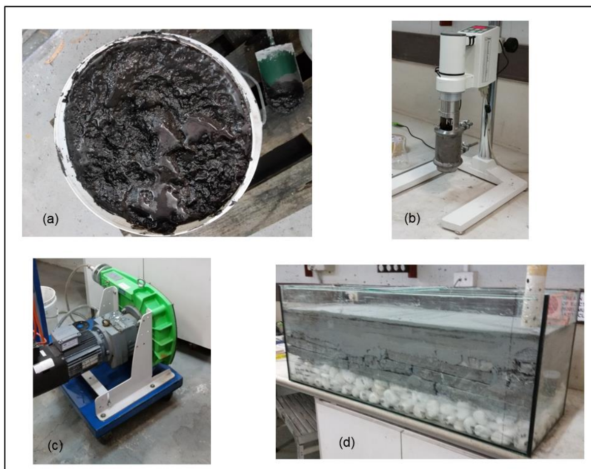
Figure 2: Experimental apparatus and materials (a) coal washery grout; (b) viscometer; (c) injection pump; (d) injection tank
