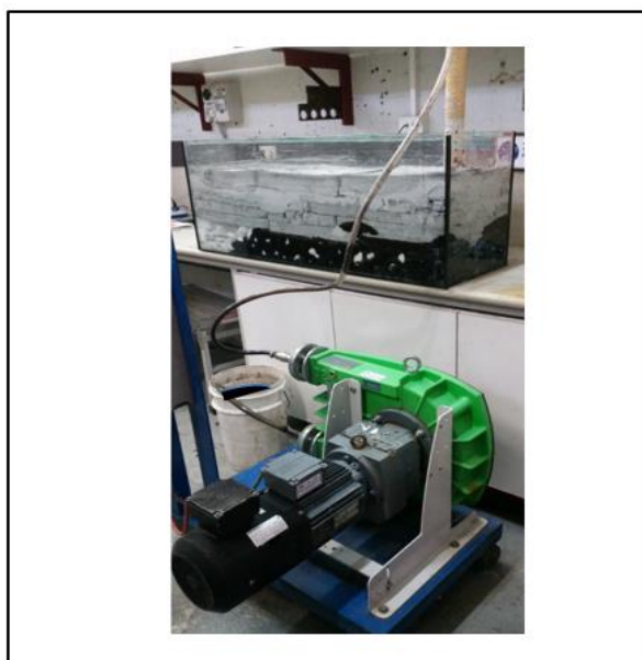
Figure 4: Connected laboratory scale injection system
