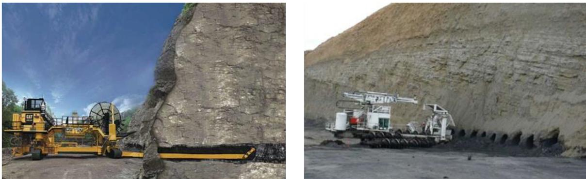
**Figure 1: Highwall mining systems (a) CHM system (after Caterpillar Inc.), (b) Auger mining system (Coal Augering Services 2014)**
