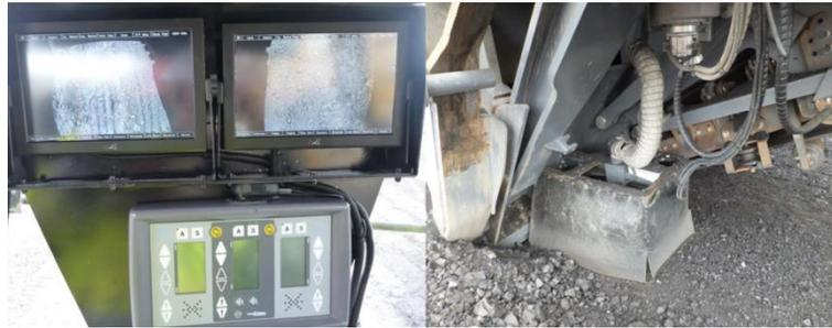
**Figure 6: Material detection camera and screen**
